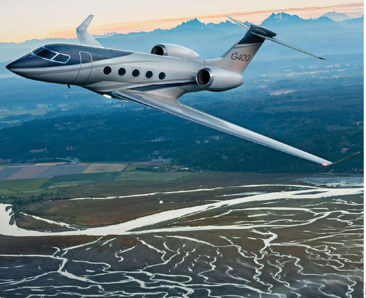
▶ PW812GA engines – certificated by Transport Canada in mid-September – each developing almost 13,500lb (60kN) of thrust. The new model will hit its maximum 4,200nm range when cruising at Mach 0.85. Maximum cruise speed will be M0.88.
